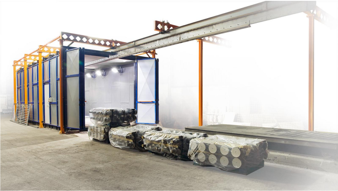
Blasting room 10x5 meters with carrier trolley and overhead C track (up to 1t), scraper floor recovery system.
