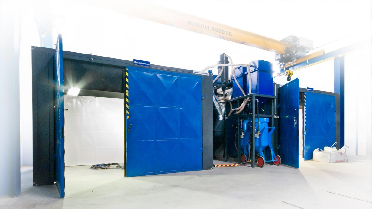
Double room 3x4 m allows blasting with two kinds of abrasives at the same time (e.g. corundum and glass beading).
