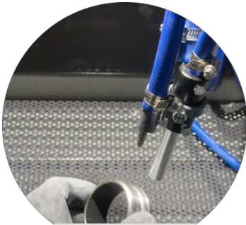
telescopic nozzle holder for comfortable blasting of small things
