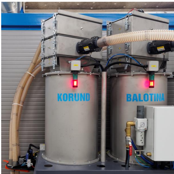
Pneumatic abrasive transport unit providing exchange of material within one blasting room. When one kind of abrasive is sucked into an appropriate reservoir the device switches from this one to another (in this case from corundum to glass beads).
