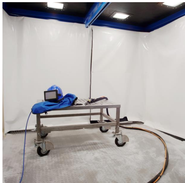
Interior with pneumatic recovery system.
