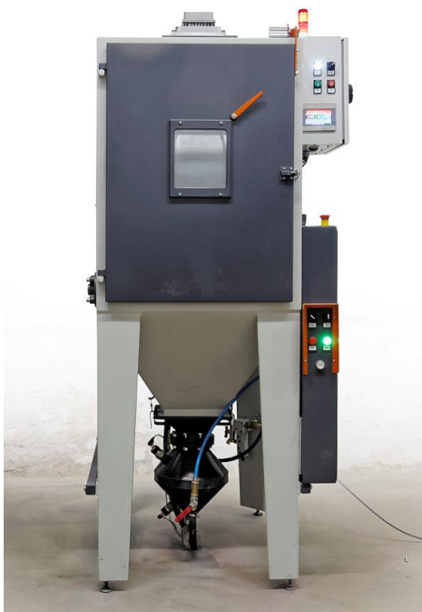
Single Tumble Blast Machine with a touch screen (pneumatic unloading)
