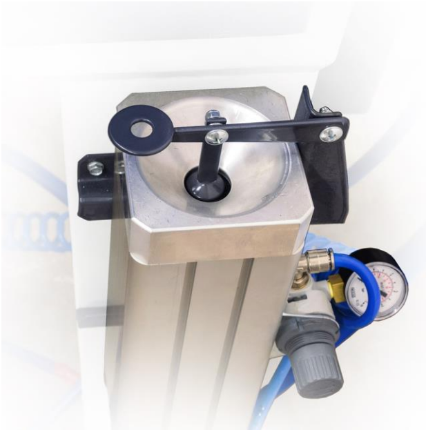
Microblaster has to be filled with new or sorted abrasive. There is a lever for filling in the picture. By pushing the lever a doze of abrasive is fed into container.
