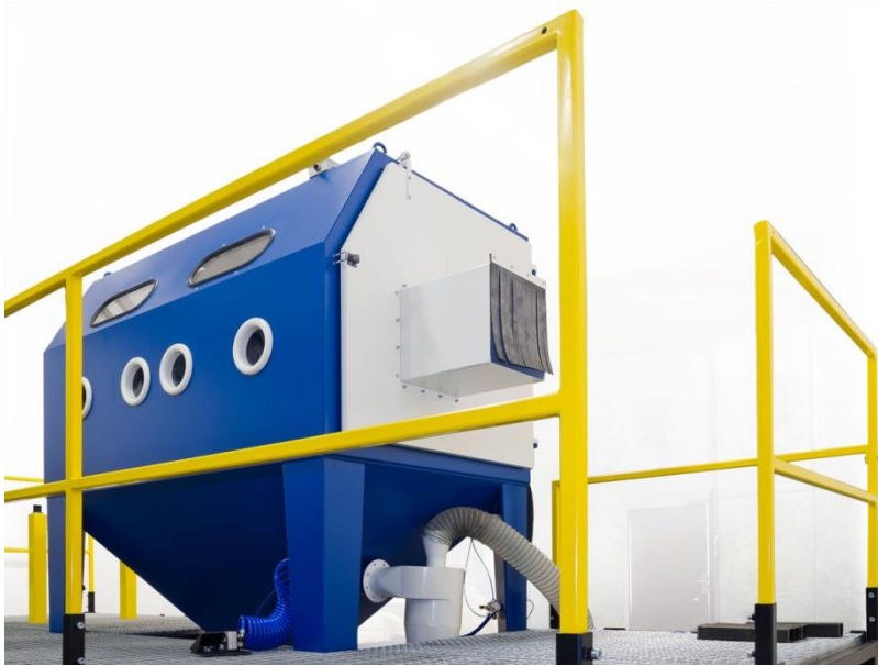
TTB 200 with working platform, draw-through openings and cyclone
