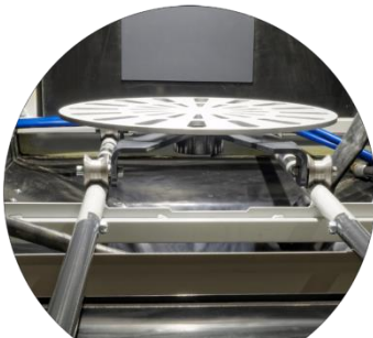
stationary or rolling-out turntable for blasting of heavy products
