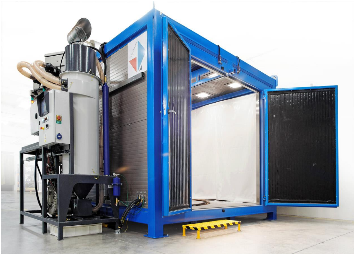
Room 3x3m with whole area suction and double external abrasive transport unit. Lever switch enables fast exchange of abrasive, e.g. corundum vs glass beads. Each abrasive has a cleaner and a reservoir of its own.
