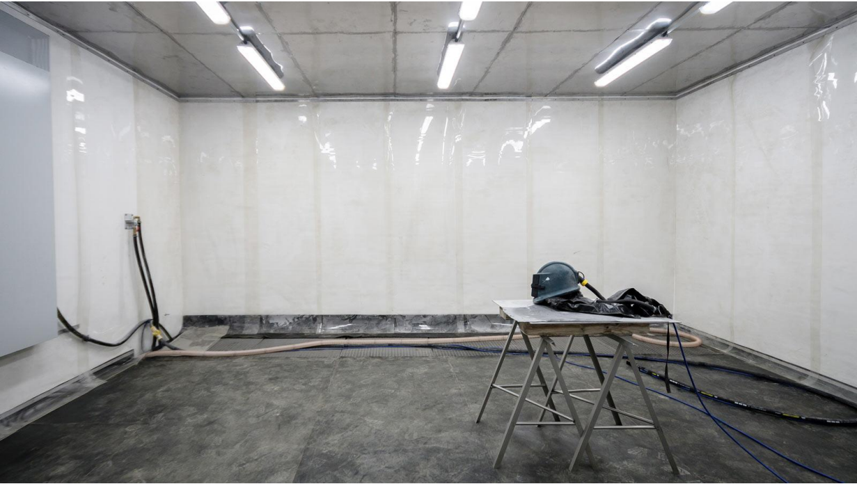
In the groove covered with grid there is a screw conveyor for mineral abrasive.
