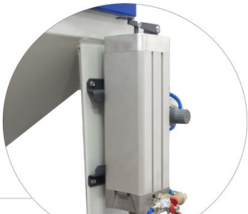
microblaster for intensive spot-blasting
